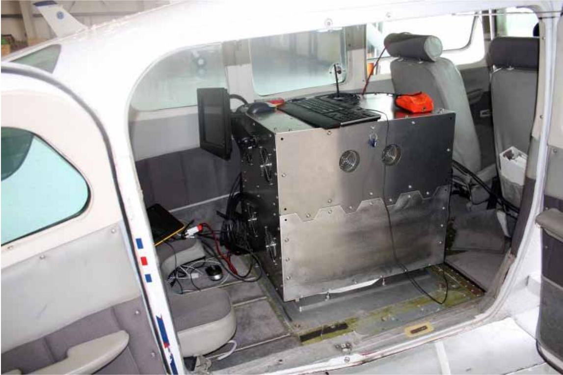
Figure 7. The Bureau's hyperspectral camera system installed in a Cessna 206.
