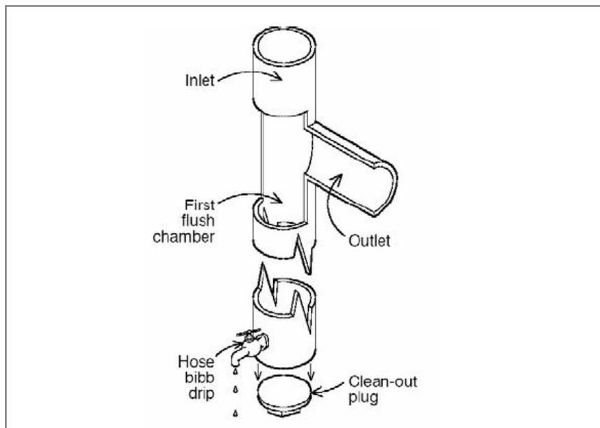
**Figure 5-24:** Standpipe first flush diverter. The recommended diversion of first flush ranges from one to two gallons of first-flush diversion for each 100 square feet of collection area. (TWDB, 2005)
