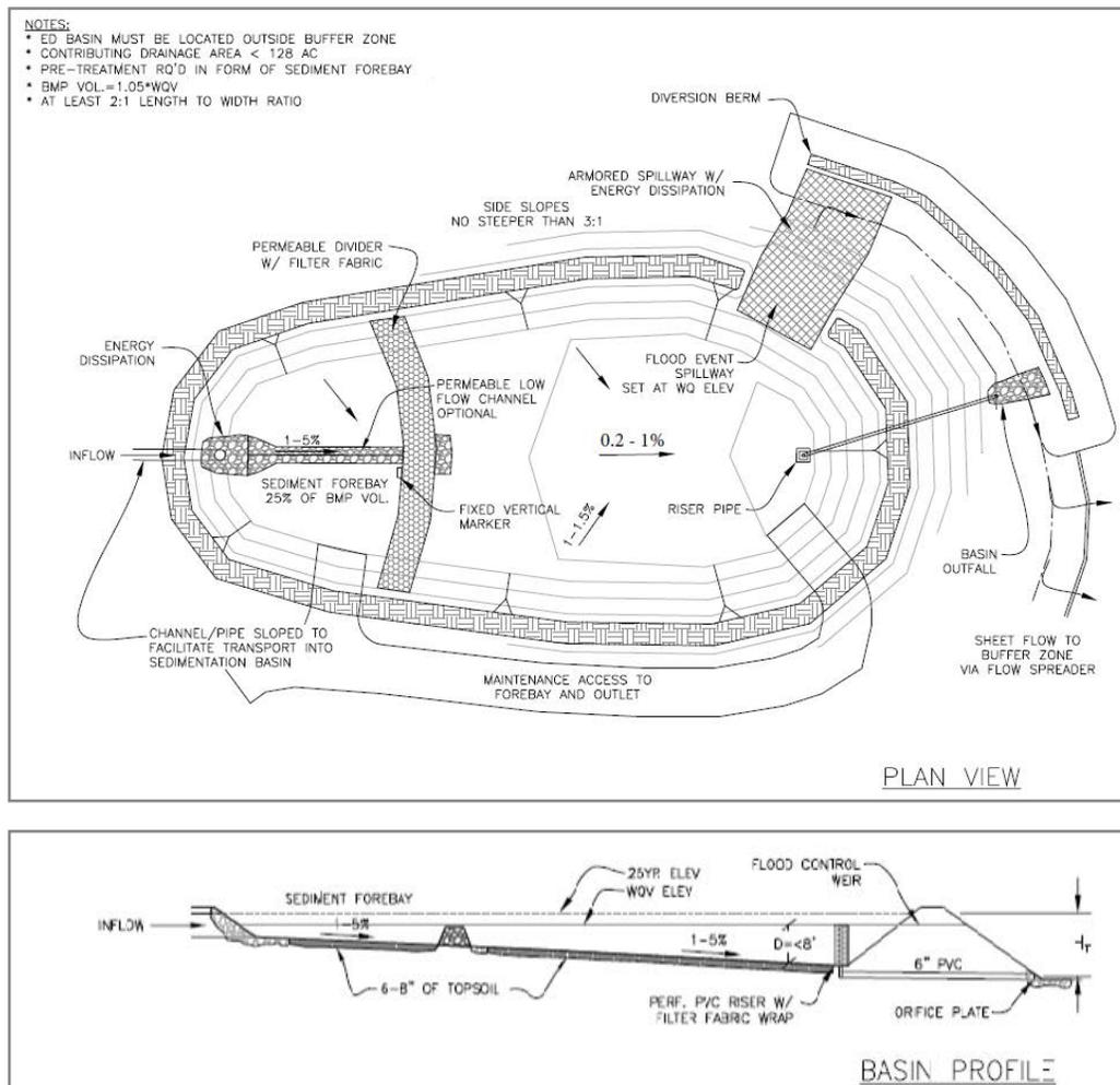
Figure 5-10: Schematic of an Enhanced Extended Detention Basin
