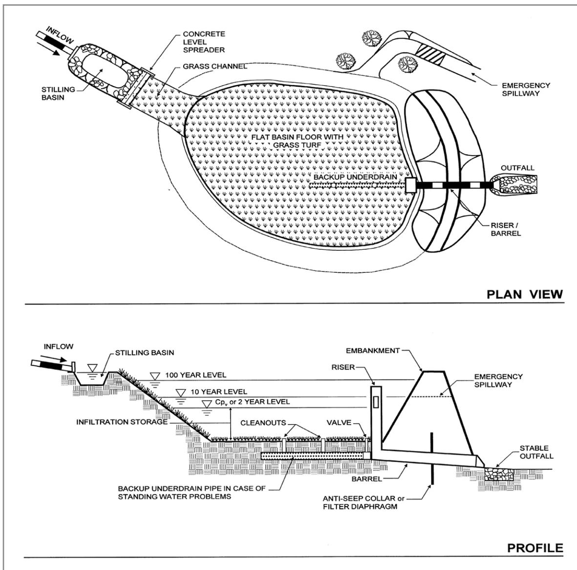
Figure 5-20: Infiltration Basin Schematic. (Photo courtesy of MDE, 2000)
