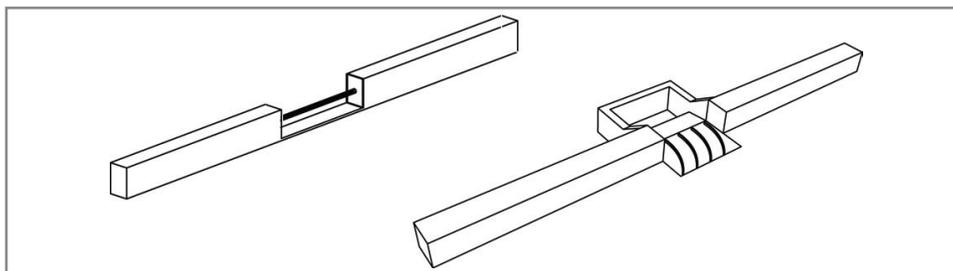
**Figure 5-17:** Curb cuts with optional sediment/trash screens.
