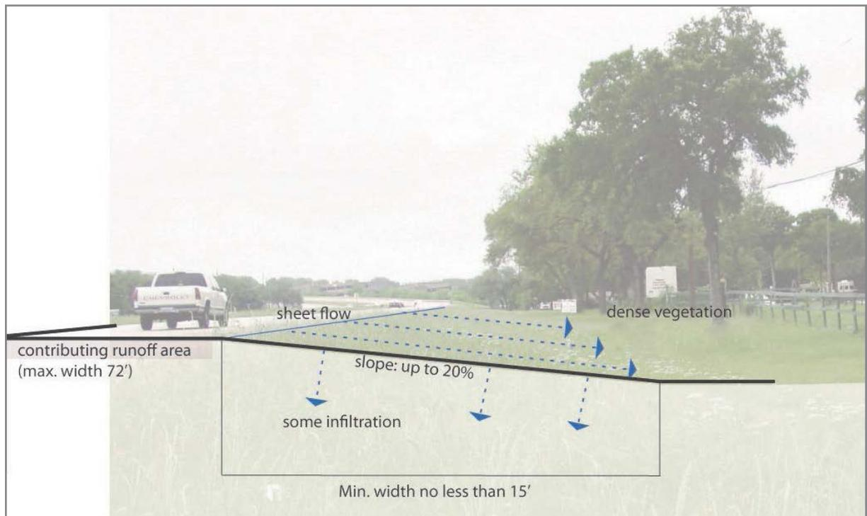
**Figure 5-3:** Filter strip along side of highway.
