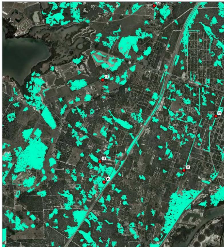
**Figure 2-1:** Depression storage in Aransas County, Texas (Larger than 1 acre in size and deeper than 2 feet).
