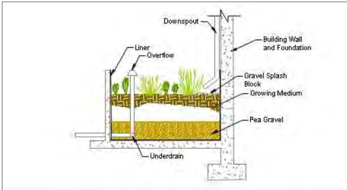
**Figure 5-19:** Stormwater Planter Box (Harris County LID Manual)
