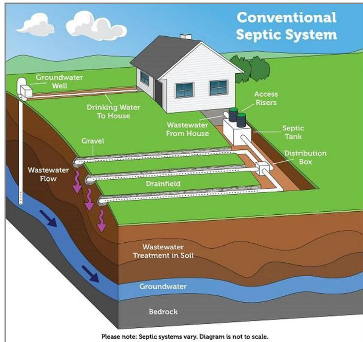
Figure 8: Schematic cut-away view of a typical septic system. Photo courtesy of US EPA.
